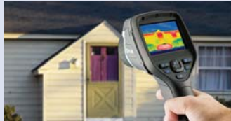
Infrared cameras quickly locate moisture related problems
