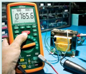
Measure the insulation resistance of transformer windings
