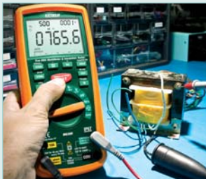
Measure the insulation resistance of transformer windings
