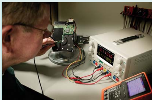
Single power supply with multiple DC outputs
