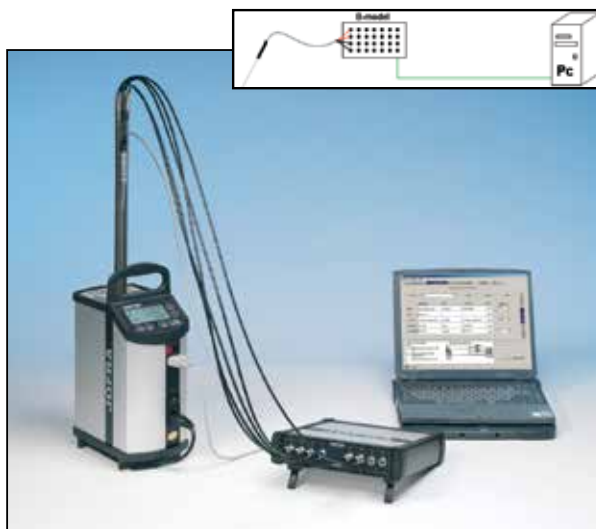
Picture 2: ASM-803 B performing its own measurements in a JOFRA ITC-320 A including an STS reference sensor in channel one all controlled by JOFRACAL.
