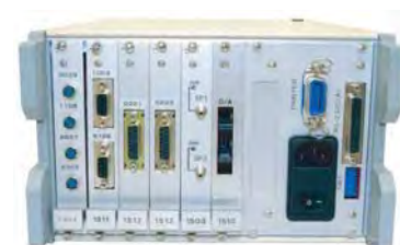
Model 1560 has 6 slots for modules
