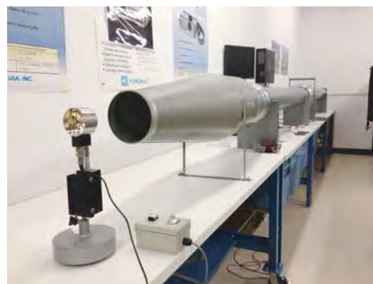
Wind Tunnel setup at Kanomax calibration lab
