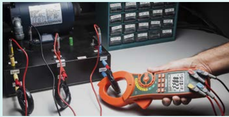
Connects to all three voltage phases simultaneously without having to move test leads from phase to phase.
