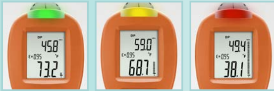
Bright LED indicator changes from green (normal, 1/3 range of Environment Temperature to Dew Point) to yellow (warning, 2/3 range which shows place will develop mildew) or red (alert, exceeds 2/3 range that shows place has mildew)
