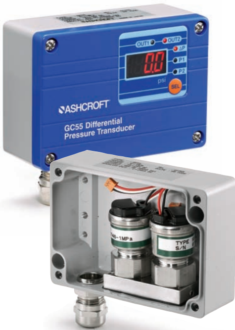
Two sensor DP design means three measurement variables in one device. Output, display and switch settings can be set in nearly ANY independent configuration to monitor, high pressure port (P1), low pressure (P2), differential (P1-P2).
