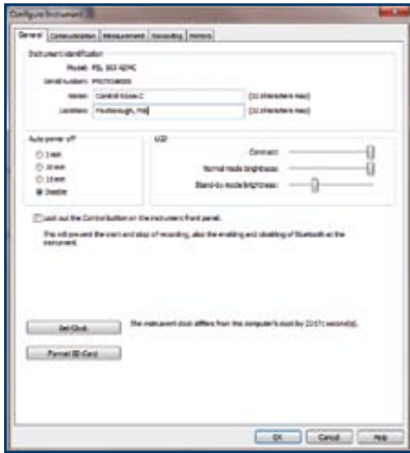
Basic information regarding Auto Power Off, instrument name and location, display brightness and contrast (Model PEL103), setting of the real-time clock and SD card formatting is easily accomplished from the General tab.
