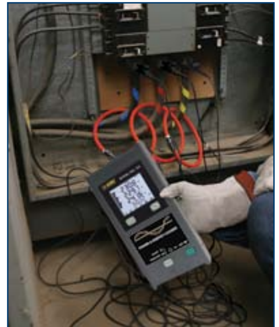
The backlit display on the Model PEL103 can be read in dark areas showing the real-time measurements.
