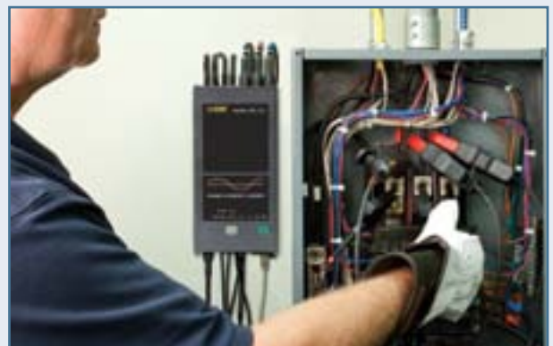
The PEL series energy loggers can safely and easily be mounted to a wall, load center panel or equipment cabinet, facilitating the connection of the voltage and current hook-ups.
